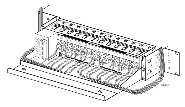
Figure 15. AVIS Chassis Cable Routing
